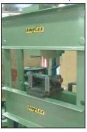
A machine shop needed to straighten forgings prior to machining. "We needed a pressing force of 100 tons and we didn't want to cut corners when it came to safety. Simplex presses do not rely on "bolt together" construction. Heavy duty pins, plus strong, welded construction across the upper bolster, puts the strength where it needs to be."
