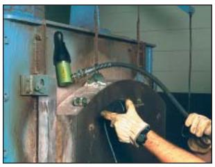
The Simplex Pow'r-Buddy™ easily provides hydraulic power to this nut splitter during routine maintenance of heat treating equipment. "Our crews have to move this equipment all around the plant; the Simplex Pow'r-Buddy™ is easy to carry and never lets us down."
