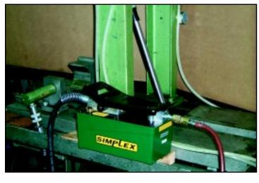
When reliable 700 bar power was needed to run this production line fixture, industrial engineers chose the Simplex PA91. "The three position treadle is easy to use and the pump runs on standard shop air."
