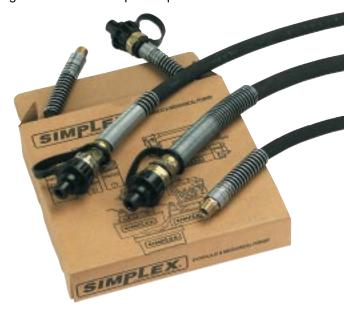
■ High Flow HD & HDC Series 3/8" I.D. hose is recommended to achieve higher retraction speeds and minimal flow restrictions. These heavy duty hoses are rated at 10,000 psi with a minimum burst pressure of 30,000 psi.
