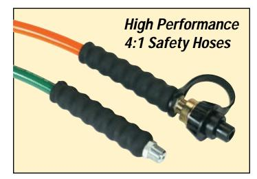
Thermo-Plastic HP & HPC Series Hoses are recommended for demanding applications. Along with their distinctive green color, the HP & HPC series hoses boast a 700 bar working, 2760 bar minimum burst, (4:1 safety factor) and a tough polyurethane outer cover that resists abrasion and wear. Well suited for continuous duty, the reinforced polyester and carbon steel wire design contributes to low volume expansion, minimized fatigue and enhanced system efficiencies.
