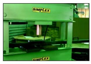
Repair personnel were faced with a variety of difficult bending, pressing, straightening and disassembly jobs. "Almost every day we have to remove bearings, straighten cylinder rods, perform wheel repair, and rebuild gear boxes. The 55 ton press is perfect; it's adjustable bed and moveable work head gives us the flexibility to work on a wide variety of jobs."
