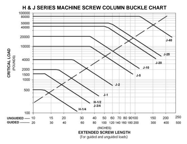
The maximum ESL values in the chart above are based on a **2:1 factor of safety against column buckle**, and on a standard design with a top plate, or a rotating design travel nut. Increased load screw lengths are not shown where the slenderness ratio exceeds 400.
