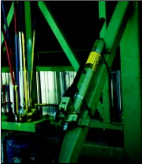
This forms manufacturer uses Simplex hand pumps and cylinders mounted to the structure for fine positioning. "We needed a hand pump that was easy to use and reliable." Simplex P41 hand pump is the preferred choice.
