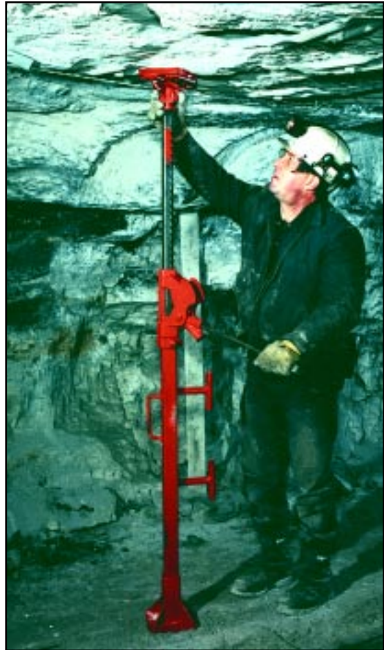
Type FS Head For support with wooden or rubber cap pieces.
