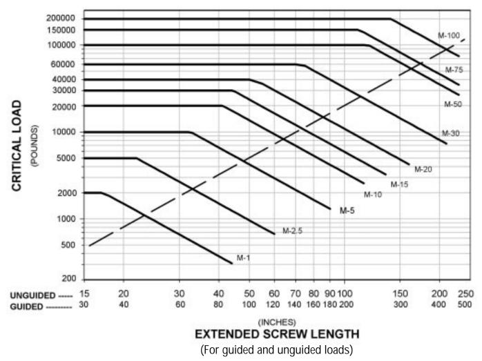
The maximum ESL values in the chart above are based on a **2:1 factor of safety against column buckle**, and on a standard design with a top plate, or a rotating design travel nut. Increased load screw lengths are not shown where the slenderness ratio exceeds 400.
