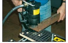
Simplex offers a punch mounted motor control, so that work can be performed safely and more productively as shown in this small fabricating shop.
