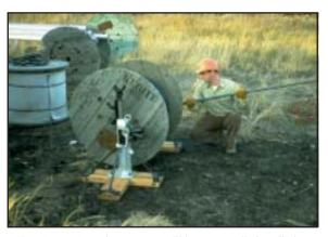
Using A1029-R and A1029-L, utilities can easily handle large reels. The large wooden bases and low handle efforts enhance safety and reduce operator fatigue. Simplex Reel Jacks are also an excellent choice for wire rope and sling manufacturers.
