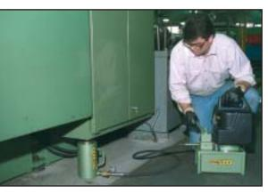
The problem was to reposition machine centers without disrupting production. "Using Simplex RLR Series cylinders and a 70 Series Suc-O-Matic pump, we rearranged our shop floor in one day." The low closed height and longer strokes eliminated extra jacking & blocking procedures, and the Simplex Suc-O-Matic valve retracted load return cylinders effortlessly.
