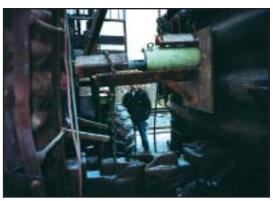
When railcar bulk heads need straightening, a 150 ton Simplex cylinder used with a SUC-O-MATIC<sup>™</sup> power pump can save the day. Simplex load return cylinders completely retract in any position when used with the Simplex SUC-O-MATIC<sup>™</sup> power pumps.
