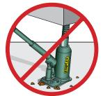
Every jack or ram whether used individually or in a system should be place on a solid, firm, non-sliding foundation so that the complete ares of its base is fully supported.
