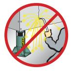
Weld splatter will damage plunger rods and hoses. Hydraulic fluid can ignite if vaporized.
