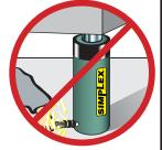
Never diconnect hydraulic hoses or fittings or couplers under pressure. Unload the ram, open the release screw on the hand pump and shift or open all hydaulic controls several times. If system includes a gauge, double check the gauge to insure pressure has been released.
