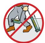
Dragging or carrying rams or pumps by a connected hose can damage the coupling and hoses. Using damaged couplers and hoses can be dangerous.
