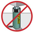
The load must be centered on the ram, or equally distributed on multiple rams. Off center loading can result in the ram slipping out and loss of the load.
