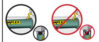
Fill pump only to recommended level. Fill only when connected cylinder is fully retracted.
