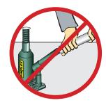
Do not use extensions or cheeter bars on hydraulic jacks or hand pumps to raise a load.
