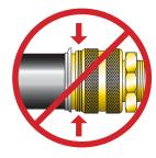
When making connections with quick couplings, make sure the couplings are full engaged. Threaded connections such as fittings, gauges, etc. must be securely tightened and leak free; however, don't use excessive force that may distort the fittings thread profile.
