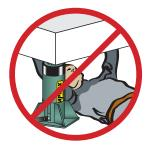
Hydraulic rams are not meant to be used as permanent supports. They are designed to lift, and lower. If you need to hold the load for any length of time cribbing or Simplex locknut cylinders should be used.
