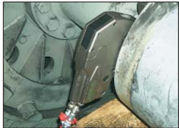
In-line reaction and compact design allows quick and easy torquing in close quarters.
