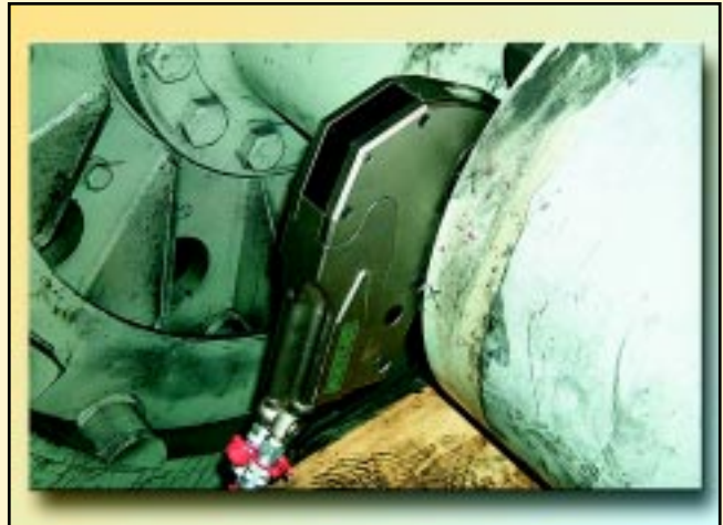
In-line reaction and compact design allows quick and easy torquing in close quarters.
