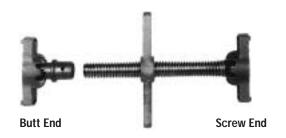
Simplex Trench Braces provide efficient, economical protection against cave-ins and costly redigging in construction and utility maintenance. Braces extend by turning the lever nut handle. The ball socket joints tilt for **added safety on angular mounting.** Holes on each end facilitate mounting to wood members.
